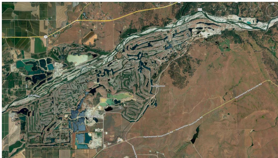
Google Earth image of the talus piles formed by dredge mining for gold along the Yuba River.
